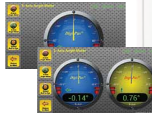
Single & Dual-Axis Angle Meter, view on smartphone or tablet screen using Digi-Pas® Level Mobile Sync Apps
