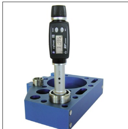
Measuring with ratchet XTD system
