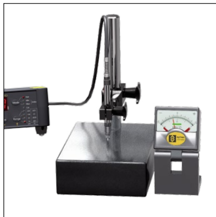
Measuring stand with P2B, D60S PRO and analog display
