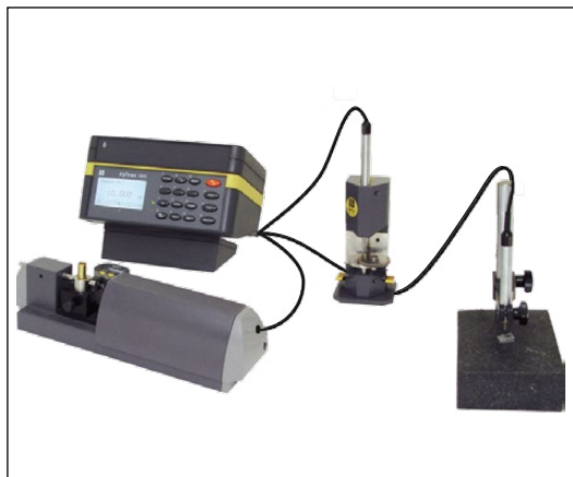
Using 3 measuring channels with 3 separated probes
