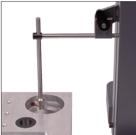
Internal groove measurement with accessories 930.2108, 930.2110 and 905.2207
