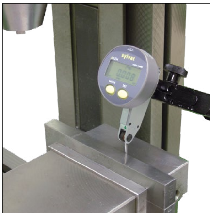
Checking the alignment on milling machine.
