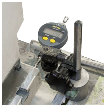
Measurent of the vertical displacement of an element
