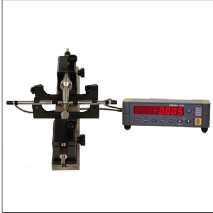
Measuring a shaft with 2 probes (A+B)
