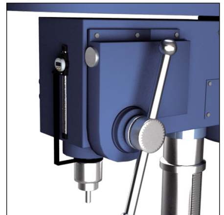
Retro-fitting on a column drilling machine with Z measuring axis
