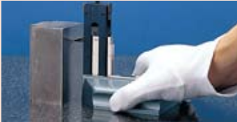
Marking a workpiece using the base, a holder and the scribe point
