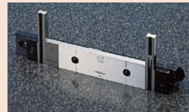
Use of B-type connectors in gage construction
