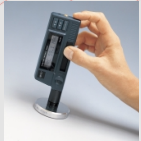
Hardness testing on a hardened work-piece
